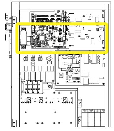
· Press down lightly on both sides of the board until two holding clips will secure the board to the support and connect the wiring signals:
