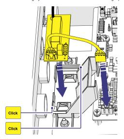
· Connec the negative pole connection cable (as in the illustration).
