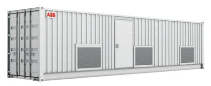
The ABB megawatt station is a compact plug-and-play solution designed for large-scale solar power generation. It houses all the electrical equipment that is needed to rapidly connect a photovoltaic (PV) power plant to a medium voltage (MV) electricity grid. All the components within the ABB megawatt station are from ABB's product portfolio.
